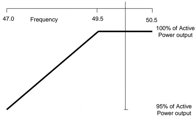
**Figure 2 – Change in output power with falling frequency**
