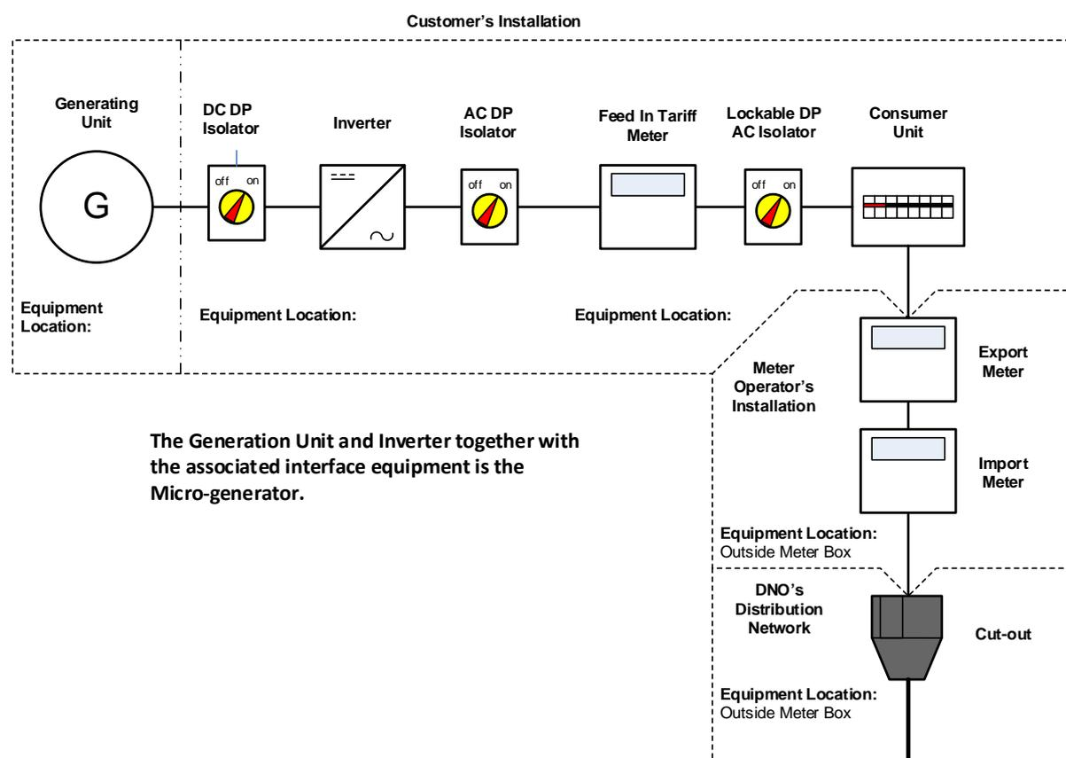
Figure 1 – Example of the type of circuit diagram
