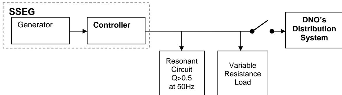
The directly coupled **SSEG** is to be tested at three levels of the directly coupled **SSEG's** output power: 10%, 55% and 100% and the results recorded on the test sheet of Appendix 4. For each test the load match is to be within  $\pm 5\%$ . Each test is to be repeated five times.
