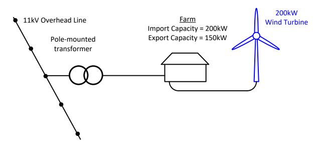
Figure E 2 - Wind Turbine Installation at a Farm
