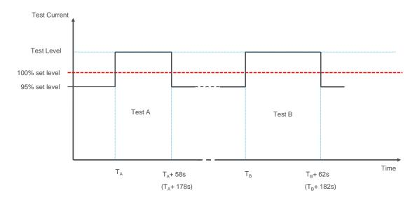
Figure 5-1 – Current Step Tests
