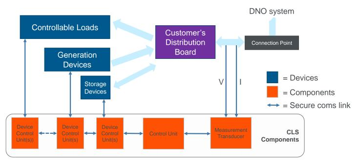
Figure 4-1 Conceptual Representation of a CLS
