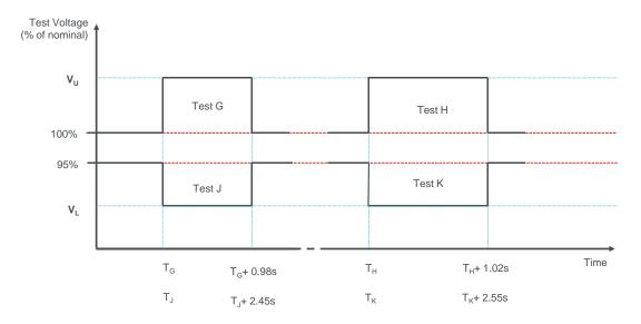
**Table 5-3 - Over and Under Voltage Tests**
