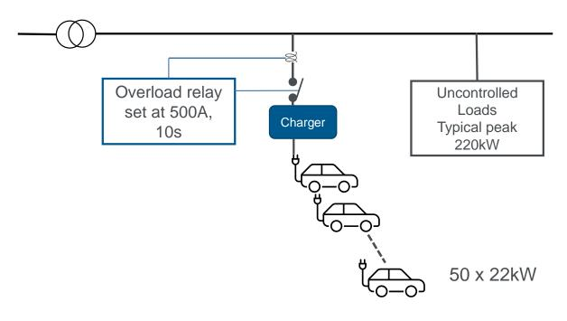
Figure E 7 Overload Protection Option (b)
