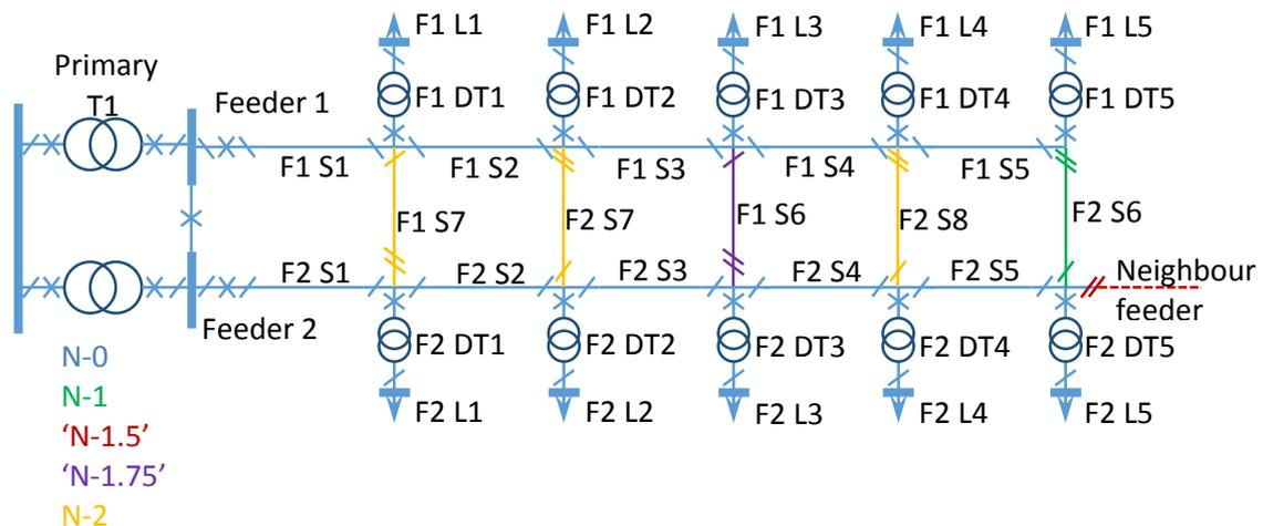
Figure 15.2: A generic HV network system with different configurations to provide certain levels of security of supply
