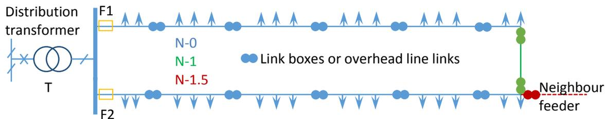
Figure 15.1: A generic LV network system with different configurations to provide certain levels of security of supply
