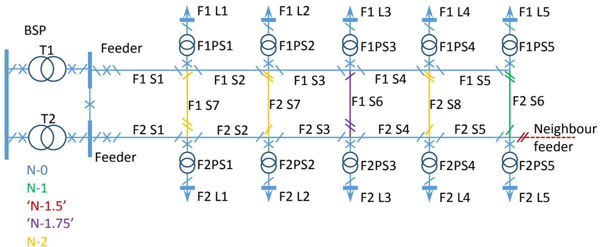
Figure 15.3: A generic EHV network system with different configurations to provide certain levels of security of supply
