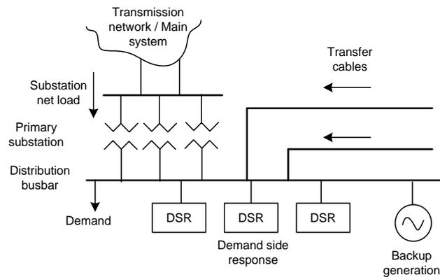
Figure 11.1: Diagram of primary substation with candidate technologies.
