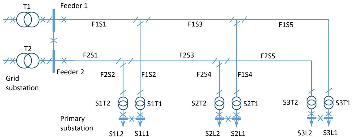
Figure 5.7: The topology of an EHV network with 3 primary substations used in the study
