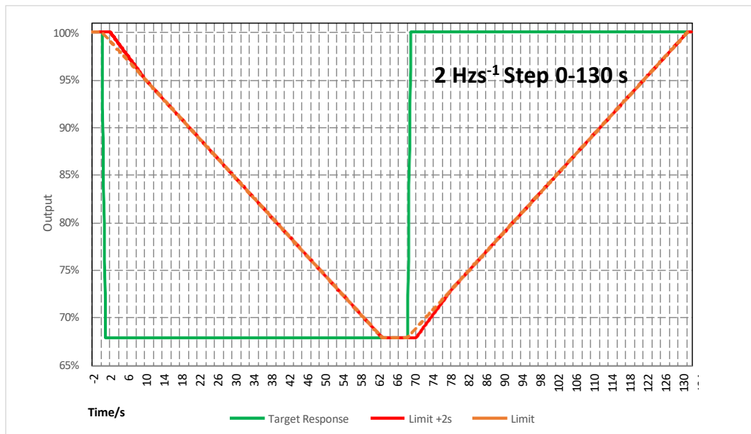
Figure B.6.1(ii): LFSM-O step response test – target response and limits
